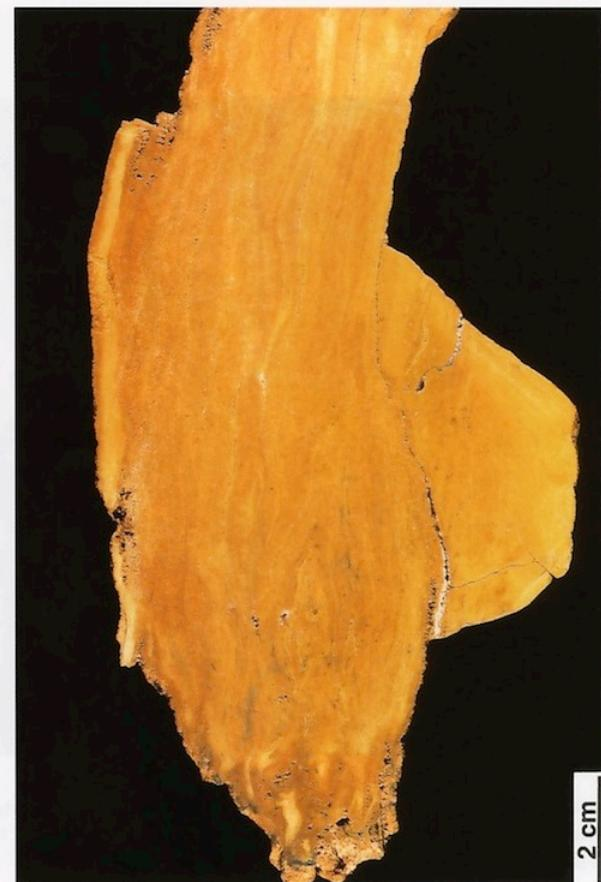
Fig. 3. Cross-section of a quartzite hand sample showing the undulately laminated structure. Laminae have thicknesses up to 1 cm.
